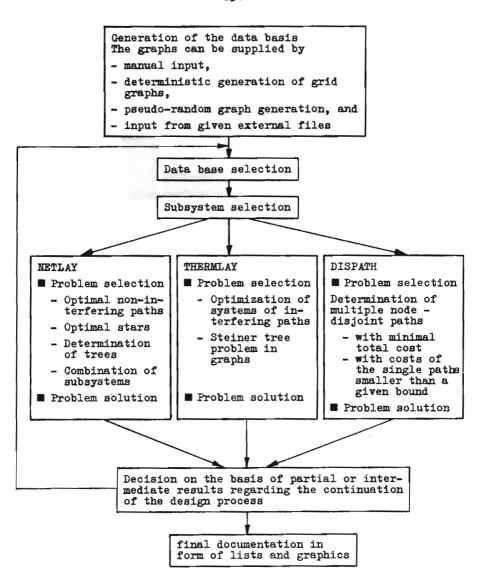
Fig. 1: Structure of program system NETOPT
